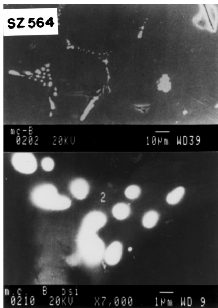
Figure 7 Secondary and backscattered electron images of SZ564 indicates 0.5% zirconia added Salem magnesite fired at 1650 °C for 4 h: (a) Showing the distribution of secondary phases in triple grain junctions; (b) an illustration of the dynamic state of ZrO_2 exsolution (1) in "suspended animation".
